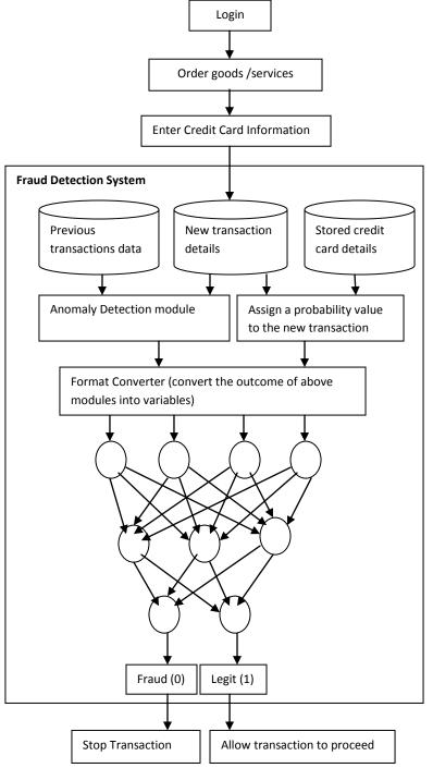
Fig. 1: Block diagram of the proposed model
